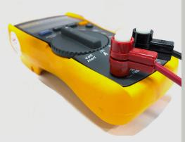
Banana plugs fit into multimeters for diagnostic testing and measurements
